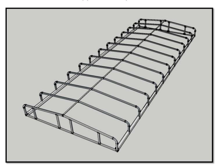
Canopy side rail lengths and the number of canopy bows will vary with the length of the Canopy. Postion the support legs to adequately cover your boat.
