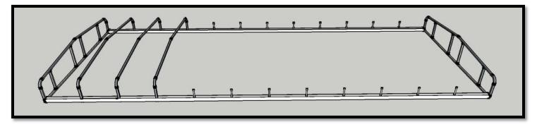
Step 4 – Lay the center strap on the top of the canopy bows. Bolt on the strap to each bow with pre-existing holes.
