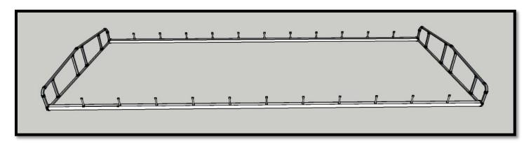
Step 3 – Push down the canopy bows on the pegs on the rail.
