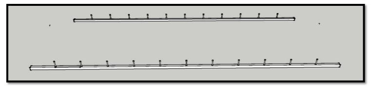
Step 2 – Slide in the end caps into the canopy rails. Then bolt them to the rails.
